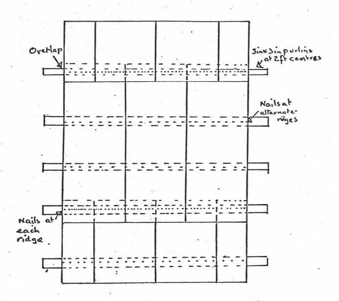
Arrangement of roof sheets for Load Testing
